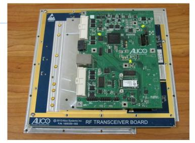
Alico Systems has developed a unique multi-functional transceiver that provides up/down conversion, digital beacon detector and back end interface options that include either a L-band IF interface or a digital interface based on LVDS. The transceiver is based on a 2 board printed circuit board assembly show above which includes the blue color RF module and green color digital controller. RF module is shielded on the top and bottom.
