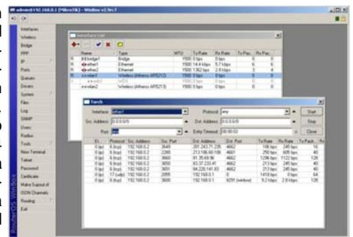
Runtime configuration and monitoring can be performed on the AP24-LFR. Some of the monitoring functions include a Wireless Sniffer to sniff packets from the wireless network, a net watch tool, and a traffic monitor tool. The traffic monitor tool is used to execute scripts when the interface traffic crosses a threshold.
