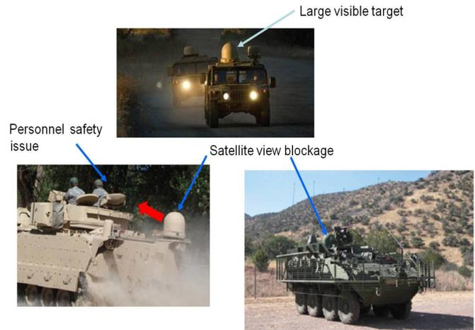
Fig. 1. Current SOTM vehicle integration concept.
