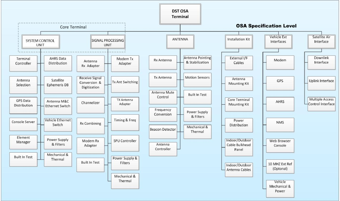
Fig. 5. DST OSA top-level functional block diagram architecture (DB = database; M&C = management and control; NMS = network management system; Rx = receive; Tx = transmit).
