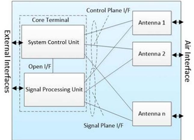
Fig. 4. DST OSA top-level block diagram architecture (I/F = interface).
