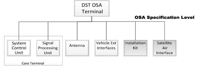
Fig. 3. DST top-level architecture.
