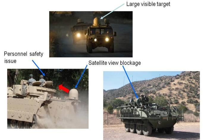
Fig. 1. Current SOTM vehicle integration concept.
